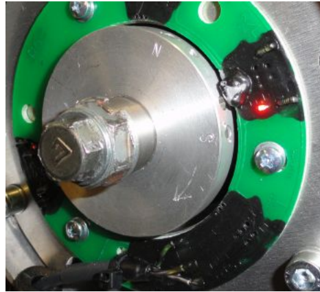
Figure 8 The LED turn on when the S-magnet passes.
