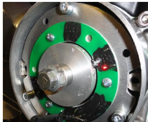
Figure 2 Mounting the magnet disk (don't tighten the set screws yet).
