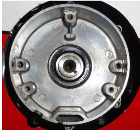
Figure 2 Removal of the old ignition components.
