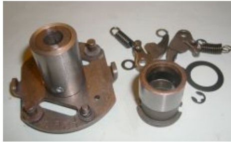
Figure 2 Removal of the old ignition components. The new driver sleeve goes over the old shaft.
