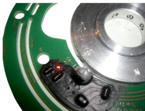
Figure 6 The LED goes on when the S-magnet passes the sensor and off when the N-magnet passes the sensor.
