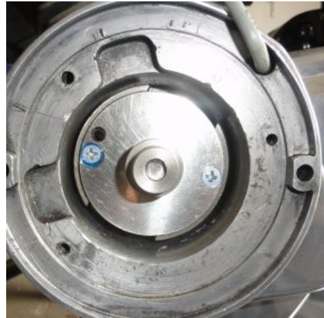
Figure 2 Mounting the driver sleeve
