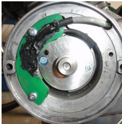
Figure 2 Mounting the pickup
