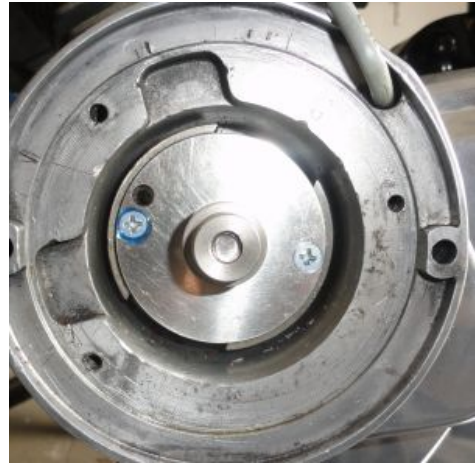
Figure 2.b Mounting the driver sleeve
