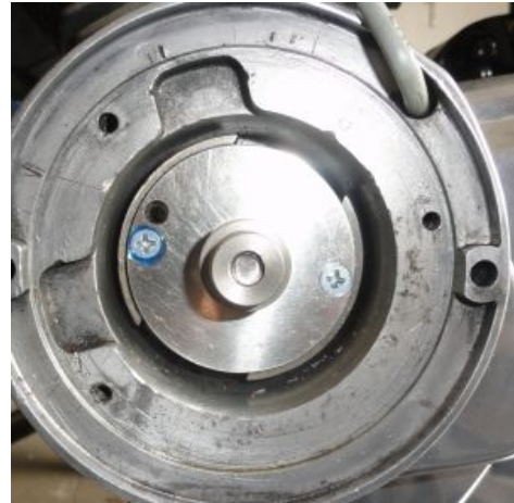
Figure 2 Mounting the driver sleeve
