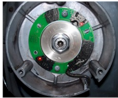
Figure 2 Complete assembly of the pickup, driver sleeve and magnet disk.
