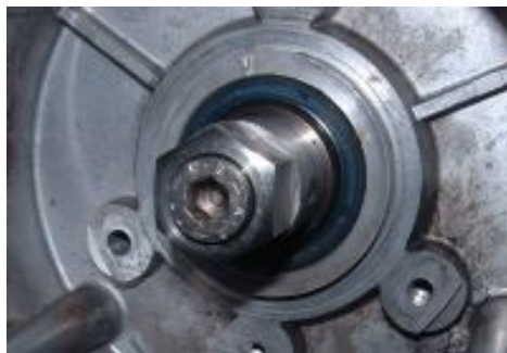
Figure 2 The driver sleeve is held in place with the centre bolt.
