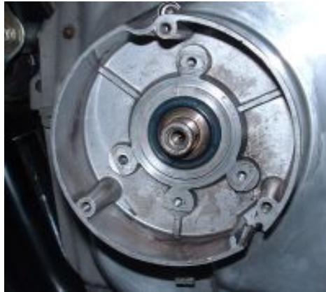
Figure 2 Removal of the old ignition components.
