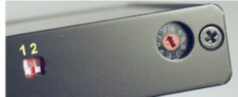
Figure 9 DIP switches and rotary switch.
