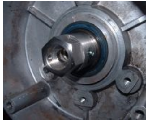
Figure 2 Mounting the driver sleeve. The set screw goes into the keyway.
