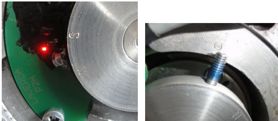
Figure 7 Initial setup and mounting the magnet disk
