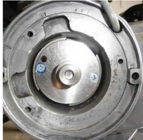
Figure 2 Mounting the driver sleeve
