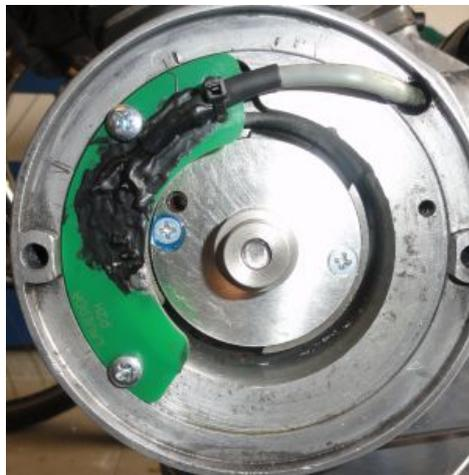
Figure 2 Mounting the pickup
