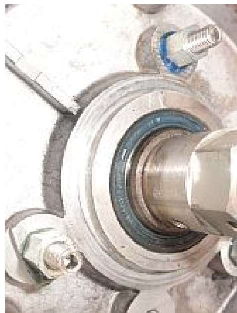
Figure 2 Spacers are put in place.
