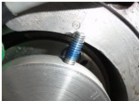
Figure 6.d Use medium strength thread lock compound for the set screws.
