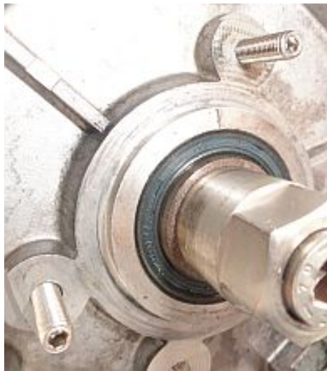
Figure 2.d The threaded rods are mounted.
