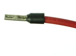
The finished crimp should look like this and not come off when pulled firmly.
