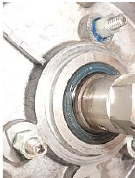
**Figure 2** Spacers are put in place.
