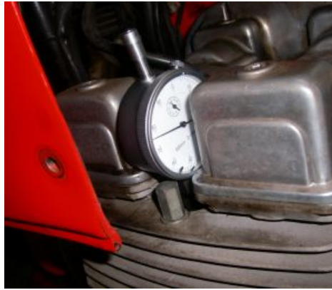
Figure 6.b Dial gauge to precisely find TDC.
