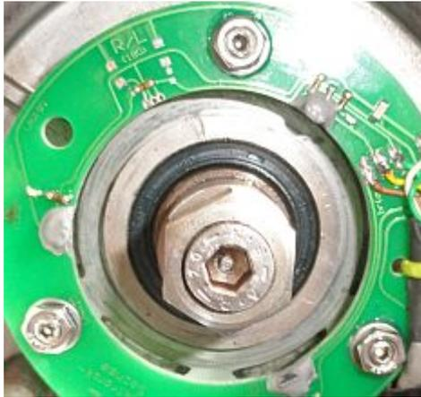
**Figure 2** The pickup is mounted.
