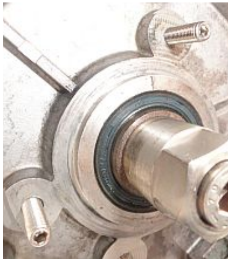
Figure 2 The threaded rods are mounted.
