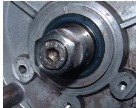
Figure 2 The driver sleeve is secured with a centre bolt.
