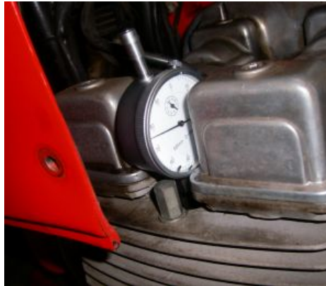
Figure 6 Dial gauge to precisely find TDC.
