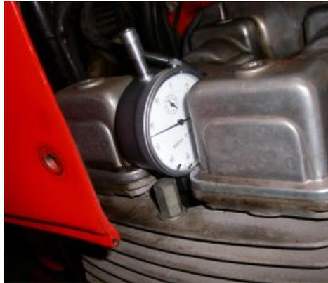
Figure 6 Dial gauge to precisely find TDC.
