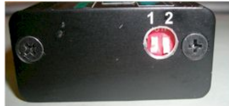
Figure 4 DIP switches and advance curve selection.
