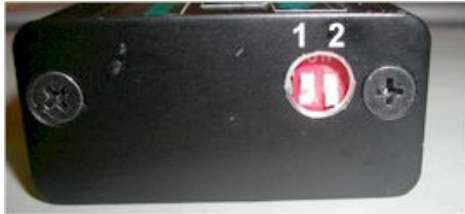
Figure 4 DIP switches and advance curve selection.
