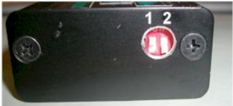
Figure 4 DIP switches and advance curve selection.
