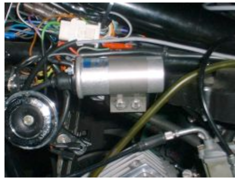
Figure 3 Mounting suggestion with PVL220 coil
