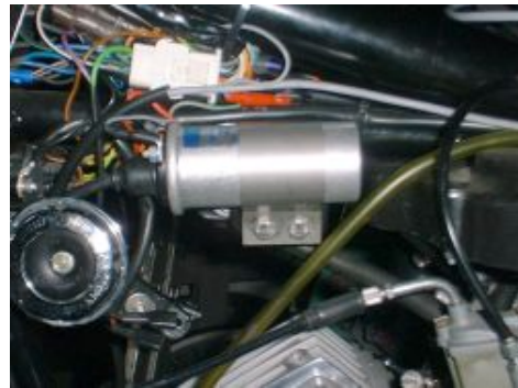
Figure 3 Mounting suggestion with PVL220 coil
