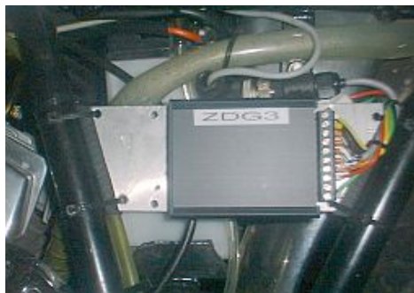
Figure 3 Mounting the ignition box
