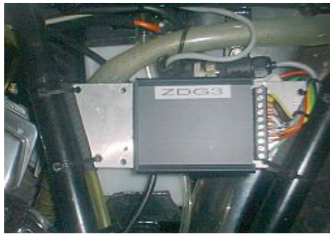
Figure 3 Mounting the ignition box
