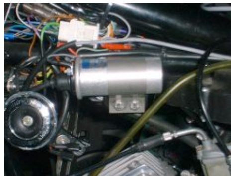
Figure 2 Mounting suggestion with PVL220 ignition coils.
