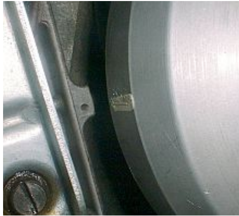
Figure 6 Set the rear piston to TDC.
