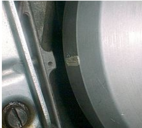
Figure 6 Set the rear piston to TDC.
