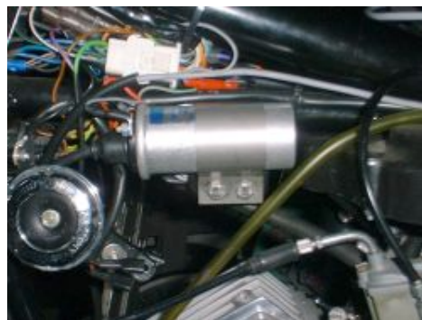
Figure 2 Mounting suggestion with PVL220 ignition coils.
