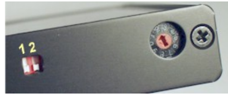
Figure 4 DIP switches and rotary switch.
