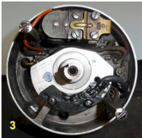
Figure 2 Mount the new pickup.
