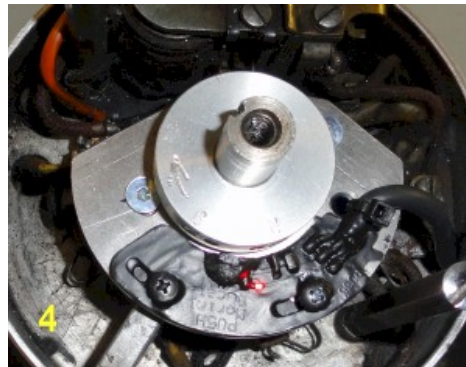
Figure 2 Mount the magnet disk on the shaft.
