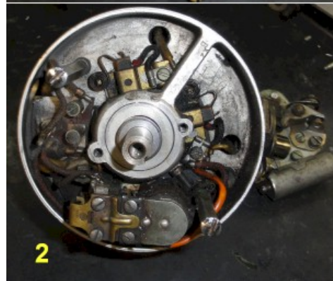
Figure 2 Remove the components of the old ignition.
