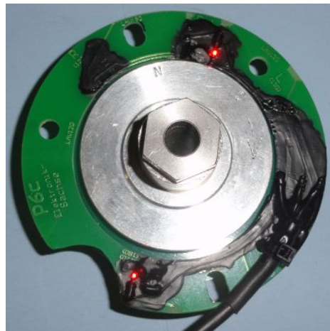
Figure 6 Pickup with driver sleeve and magnet disk.
