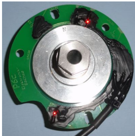
Figure 6 Pickup with driver sleeve and magnet disk.
