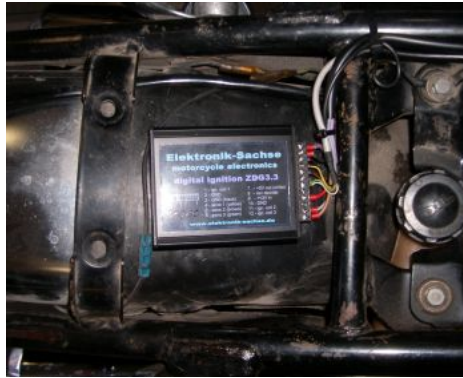
Figure 3 Mounting suggestion of the ignition box.
