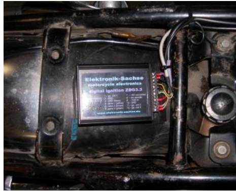
Figure 3 Mounting suggestion of the ignition box.
