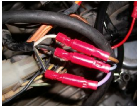
Figure 5 Coil cable connection.
