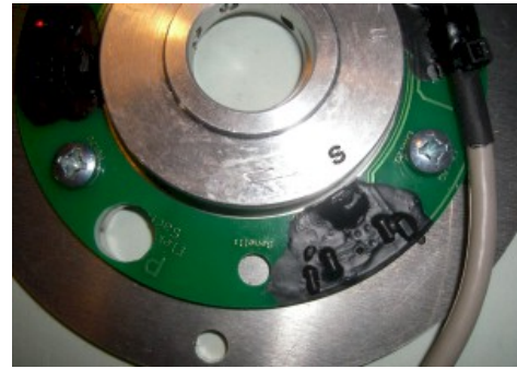
Figure 8 The LED goes off when the piston is on TDC.
