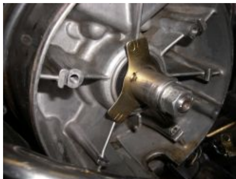
Figure 2 Removal of the old ignition components.
