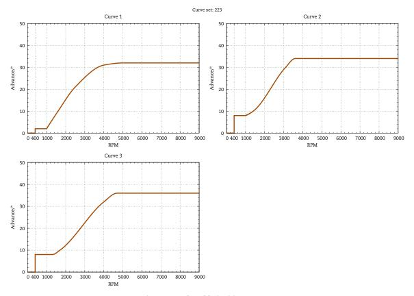
Figure 6 Selectable ignition curves.
