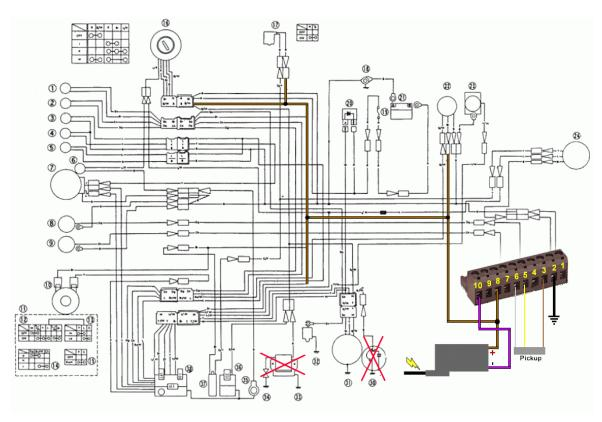
Complete diagram. Note the shipped terminal connector actually has six connections instead of the ten displayed here.
