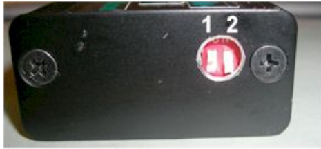
Figure 5 DIP switches and advance curve selection.
