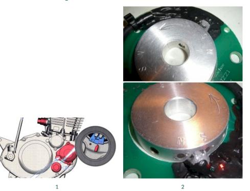
If the magnet disk happens to have two pairs of N and S magnets, it doesn't matter which pair is used for the initial setup. It is also not relevant which TDC (compression stroke or exhaust stroke) is used for the initial setup.
