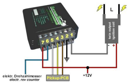
Wiring schematic with dual output coil.
