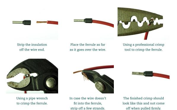
Figure 3 Crimping the wire end ferrules.
