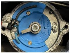
Figure 2 Removal of the old ignition components. Guzzi pickup.
