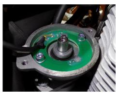
Figure 2 Mount the pickup.
