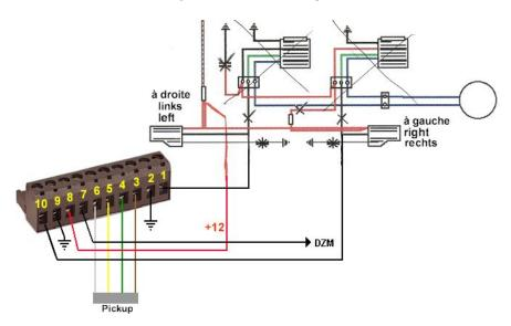
Figure 4 Connection in the original wiring. Motoplat replacement.
