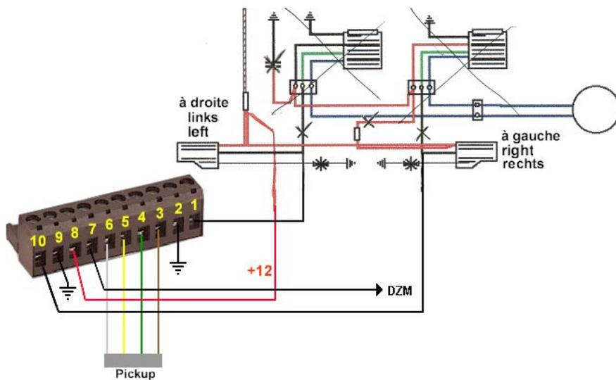
Figure 4 Connection in the original wiring. Motoplat replacement.
