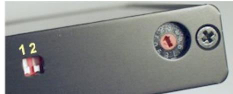
Figure 8 DIP switches and rotary switch.
