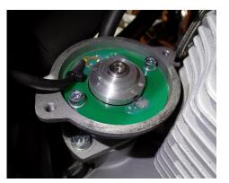
Figure 2 Final assembly of pickup and magnet disk.
