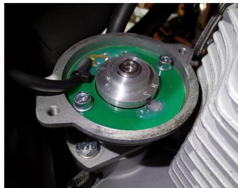
**Figure 2** Final assembly of pickup and magnet disk.
