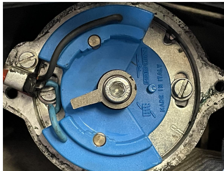
Figure 2 Removal of the old ignition components. Guzzi pickup.
