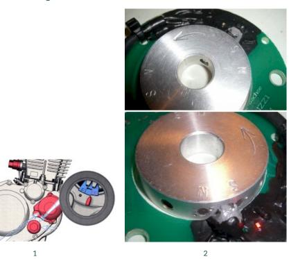
If the magnet disk happens to have two pairs of N and S magnets, it doesn't matter which pair is used for the initial setup. It is also not relevant which TDC (compression stroke or exhaust stroke) is used for the initial setup.
