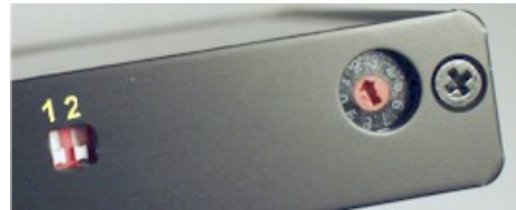
Figure 5 DIP switches and rotary switch.
