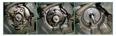
Figure 2 Remove the original contact breaker plate and the advance unit
