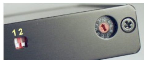
Figure 7 DIP switches and rotary switch.
