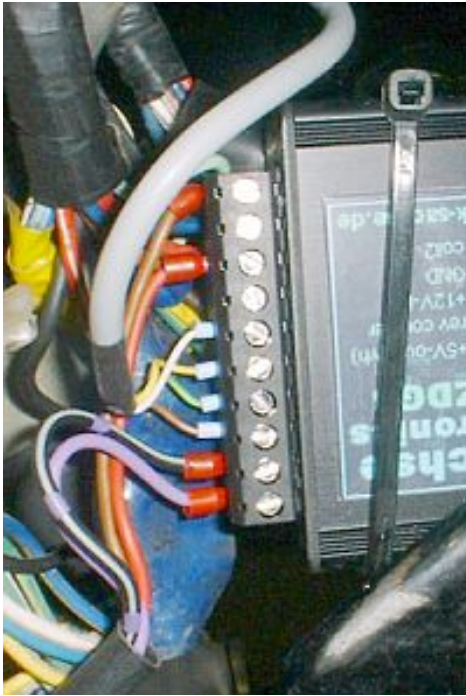
Mounting of the ignition box
