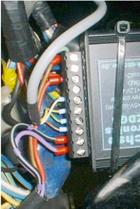
Mounting of the ignition box
