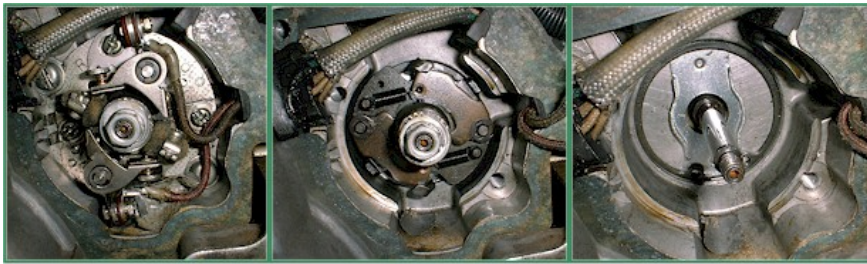
Figure 2 Remove the original contact breaker plate and the advance unit
