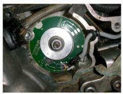
At last put the magnet disk onto the sleeve hub, but do not tighten the set screws yet.
