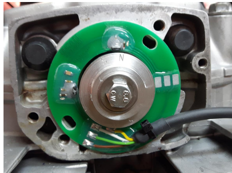
Pickup with driver sleeve and mounted magnet disk. The pickup has not yet been fixed with the M5 screws.
