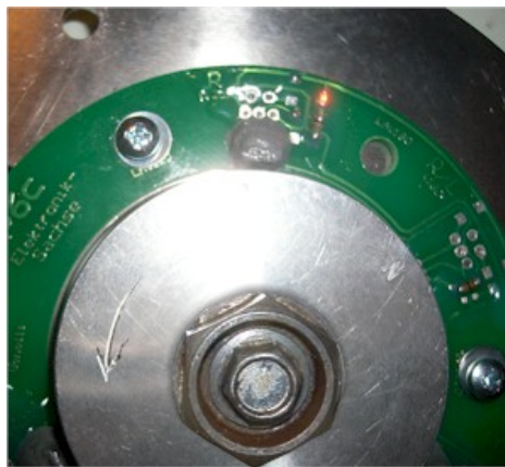
Figure 8 When the S-magnet passes, the LED turns on.
