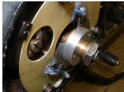
Figure 2 Alignment of the magnet disk to the sensors (note that the image shows an older version).
