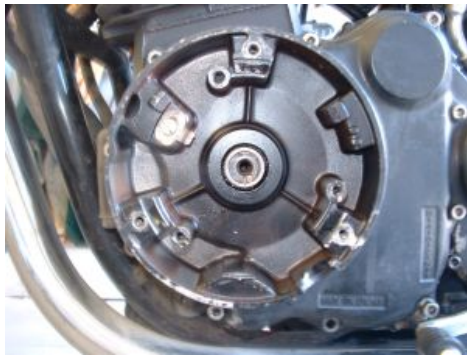
Figure 2 Removal of the old ignition.
