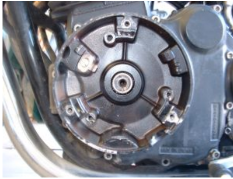
Figure 2 Removal of the old ignition.
