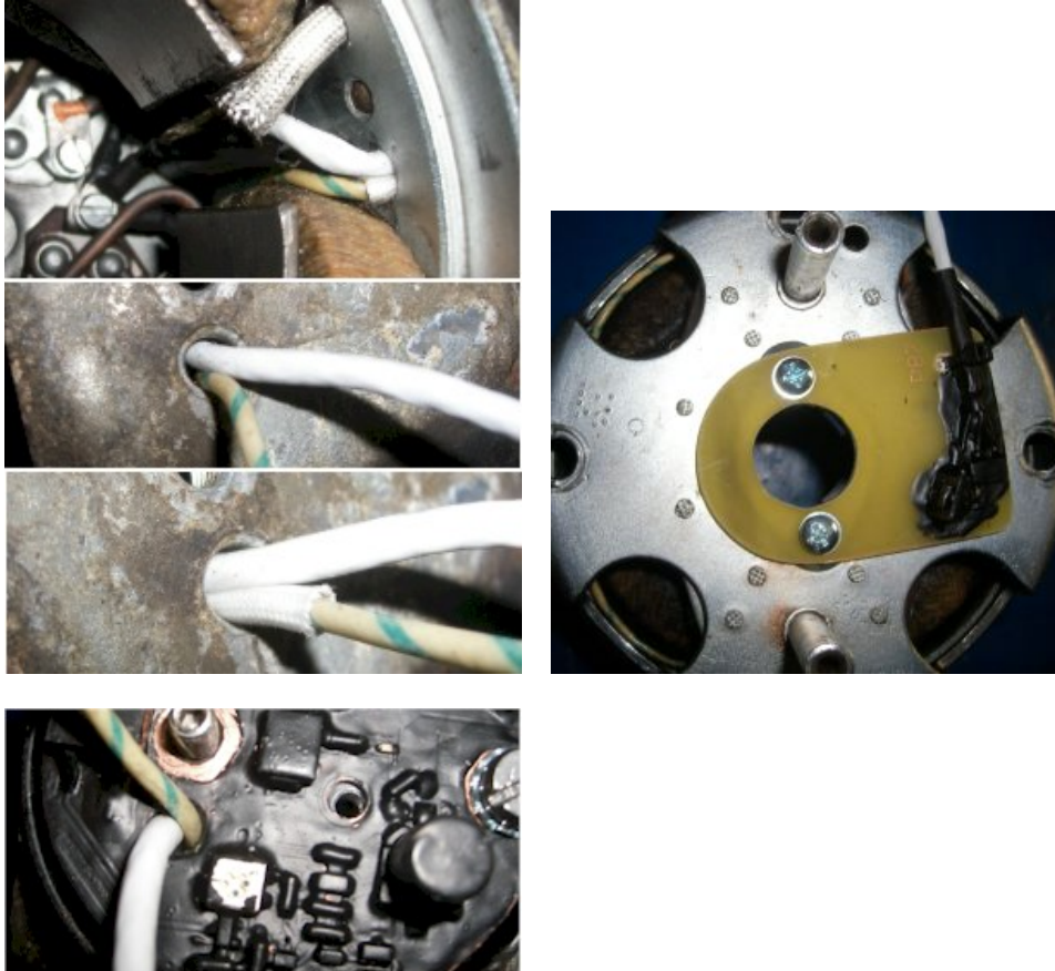
Cable routing through the regulator base plate (in this picture the regulator RegKS is shown)
