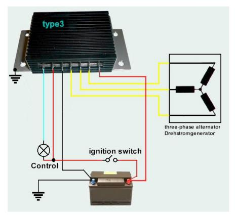
Figure 2 General schematic of how the regulator is connected.
