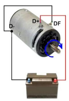
Test circuit for regulator REG5a.
