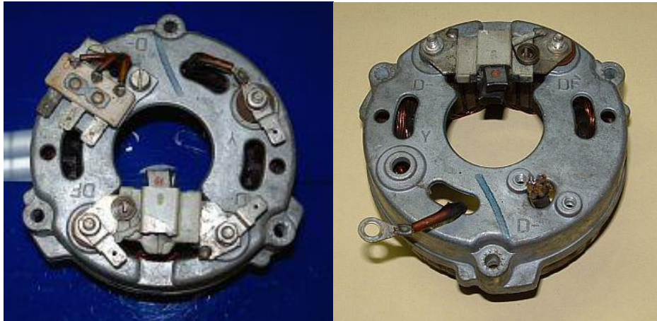
Figure 1 Remove the connector block and Y-connection.
