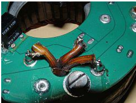
Figure 3 Solder the three wires from the alternator
