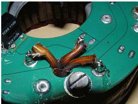
Figure 3 Solder the three wires from the alternator
