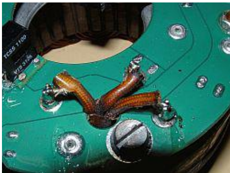
Figure 3 Solder the three wires from the alternator
