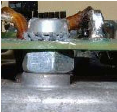
Figure 2 Use the nut as spacer
