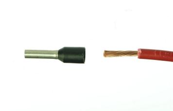
Strip the insulation off the wire end.
