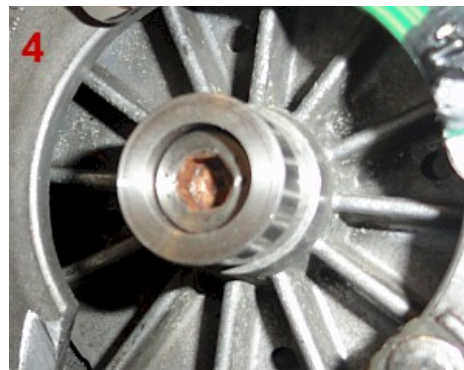
Mounting the drive sleeve hub
