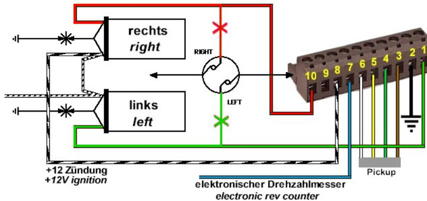
Figure 3 Ignition circuit diagram, breaker points replacement
