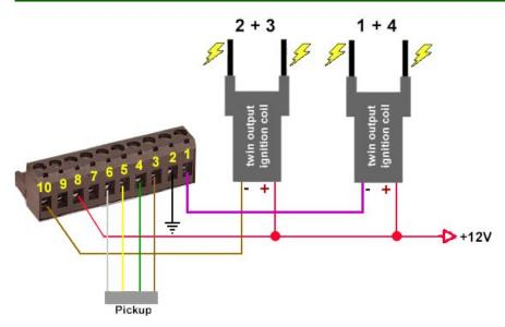
Connection with the wiring diagram
