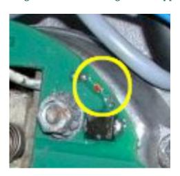
Figure 12 LED for the regulator circuit.
