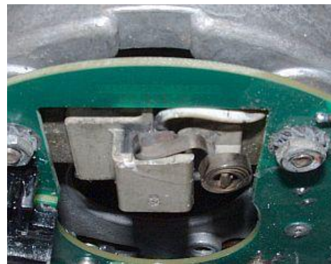
Figure 5 Unclip the brusher spring
