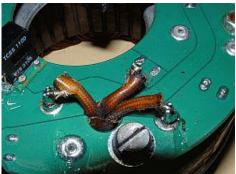
Figure 4 Solder the three wires from the alternator.
