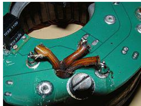
Figure 4 Solder the three wires from the alternator.
