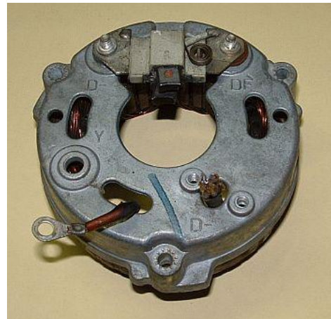
Figure 2 Remove the connector block and Y-connection.
