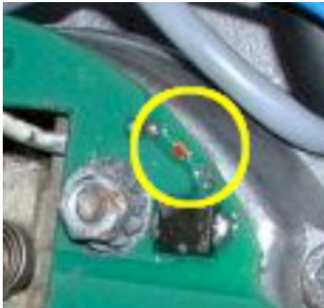
Figure 12 LED for the regulator circuit.
