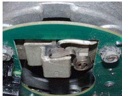
Figure 5 Unclip the brusher spring
