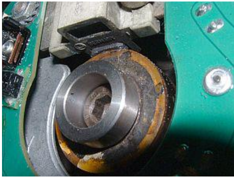
Figure 7 Mounting of the stator and driver sleeve
