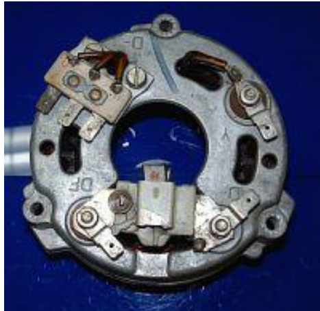
Figure 2 Remove the connector block and Y-connection.
