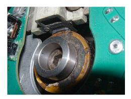
Figure 7 Mounting of the stator and driver sleeve
