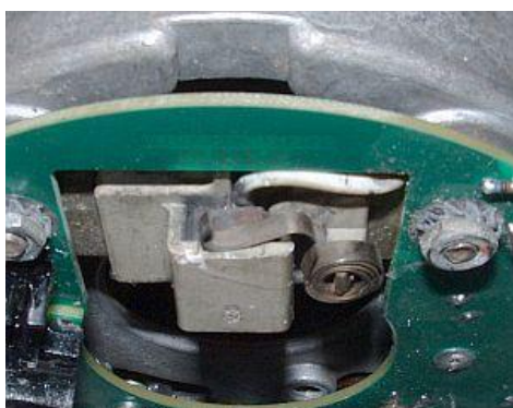
Figure 5 Unclip the brusher spring
