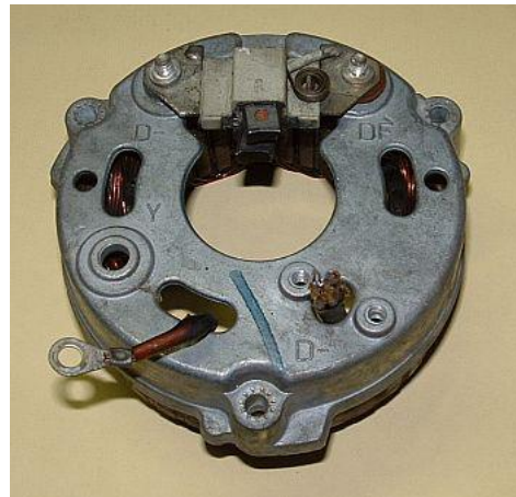
Figure 2 Remove the connector block and Y-connection.
