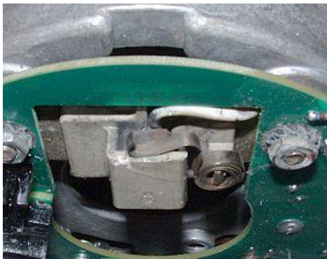
Figure 5 Unclip the brusher spring
