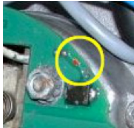
Figure 12 LED for the regulator circuit.
