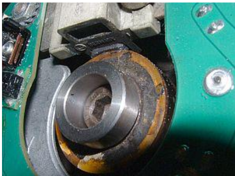
Figure 7 Mounting of the stator and driver sleeve
