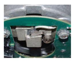
Figure 5 Unclip the brusher spring
