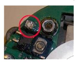
**Figure 17** Trimmer to select charging voltage.
