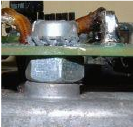
Figure 3 Use the nut as spacer.
