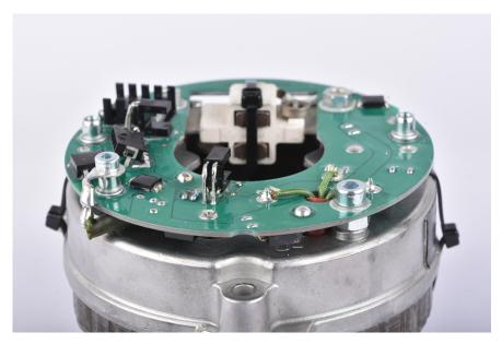
Figure 6 The mounted regulator
