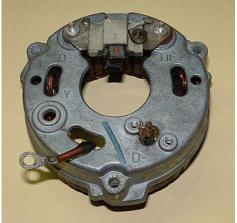
Figure 2 Remove the connector block and Y-connection.
