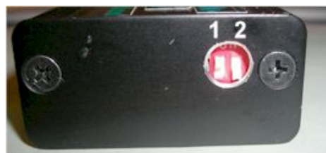
Figure 4 DIP switches and advance curve selection.
