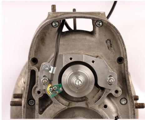
Put the magnet disk on the sleeve hub. But don't tighten the set screws, yet.
