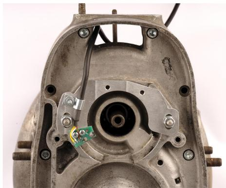
Fix the pickup base plate using the threaded rods and the M6 nuts. Centre it using the slotted holes, so it can be slightly adjusted to either side if required.
