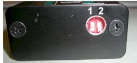
**Figure 5** DIP switches and advance curve selection.
