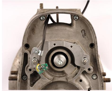
Secure the sleeve hub with the M8 screw and the serrated washer.
