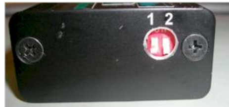
Figure 5 DIP switches and advance curve selection.
