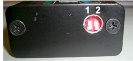
Figure 5 DIP switches and advance curve selection.
