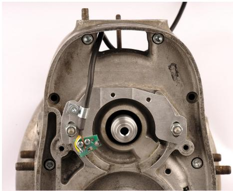
Then place the sleeve hub on the cam shaft. The taper should fit perfectly. Adding a bit of oil to the sleeve hub helps pushing it in place more easily.
