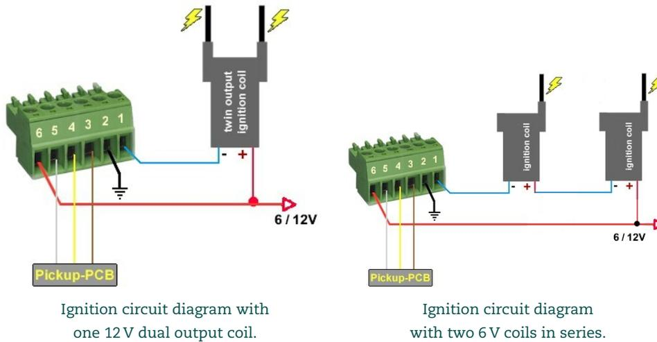
Ignition circuit diagram with one 12 V dual output coil.
