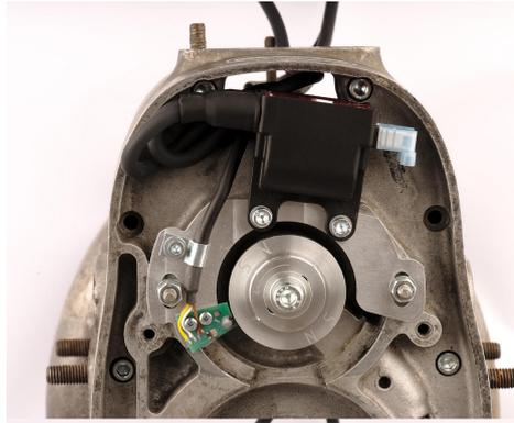
Install the ignition coil with the provided M5 screws. Make sure you use thread locking compound for the screws. Alternatively the coil can be mounted outside the engine. The latter option offers better cooling.
