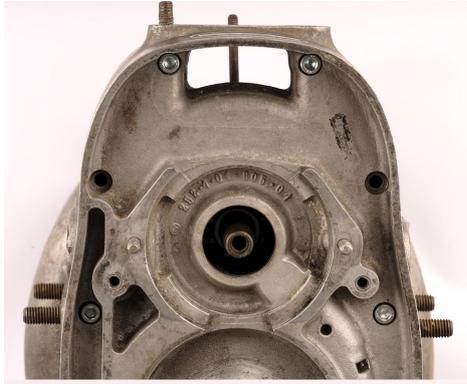
Take off the original parts, so only the cam shaft remains. That includes the original ignition, points, weights, condensers and manual advance mechanism.
