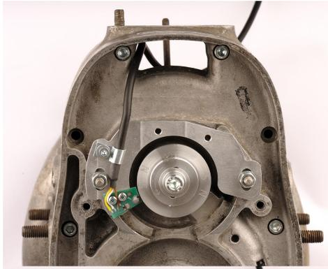
Put the magnet disk on the sleeve hub.
