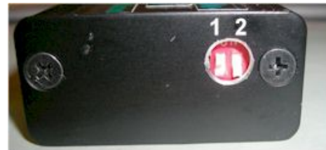
Figure 5 DIP switches and advance curve selection.
