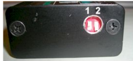
Figure 5 DIP switches and advance curve selection.
