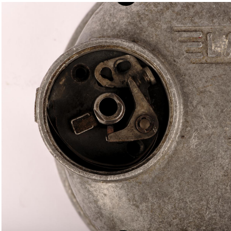
Remove the ignition cover.
