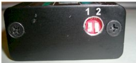
Figure 4 DIP switches and advance curve selection.
