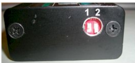
Figure 4 DIP switches and advance curve selection.
