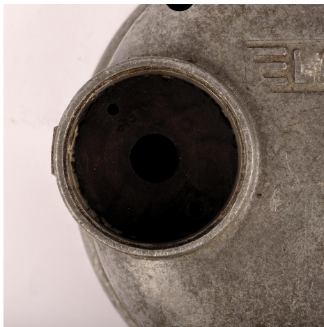
Remove the breaker points and the original weights advancer.
