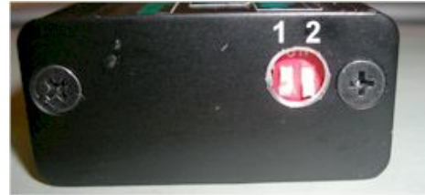
Figure 4 DIP switches and advance curve selection.
