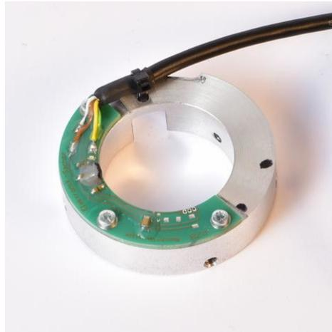
This is the new pickup including the base plate that will now be mounted in the distributor housing.
