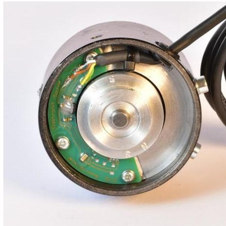
Now the magnet disk is mounted. The set screws don't need to be tightened just yet. The disk is just placed loosely on the shaft. It will be tightened at a later point.
