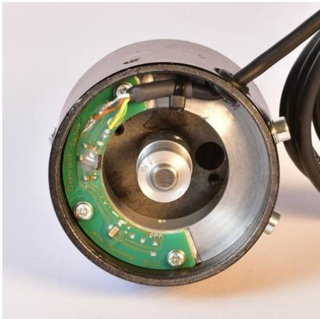
The pickup base plate is mounted and fixed with the M4 screws. The connection lead is run through the existing hole in the distributor. A grommet is required to protect the lead from the sharp corners.
