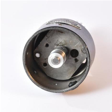
Remove the lid and the old parts of the ignition. The points and weights are not required any longer. What remains is an empty distributor housing with the shaft. Now mount the new driver sleeve on the shaft and secure it with the set screws.
