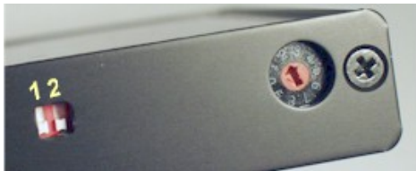
Figure 4 DIP switches and rotary switch.
