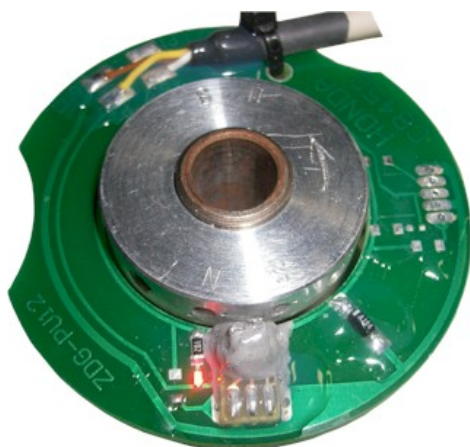
Figure 3 Ensure correct alignment of magnet disk and sensor.
