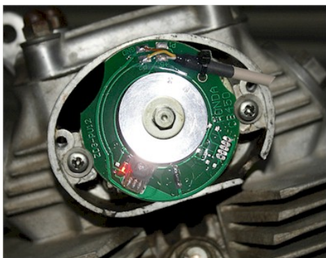
Fitting of the sensor plate (photomontage)
