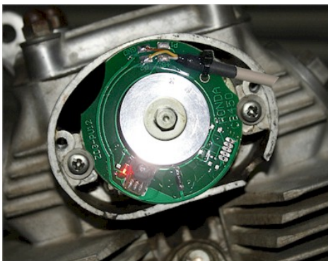
Fitting of the sensor plate (photomontage)
