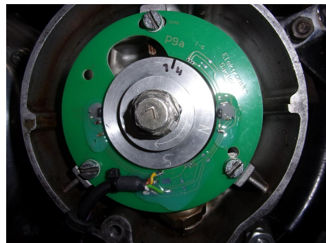
Figure 2 Mounting the new pickup, driver sleeve and magnet disk. The set screws in the magnet disk need not be tightened at this point, yet.
