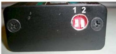
Figure 4 DIP switches and advance curve selection.
