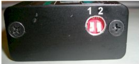
Figure 8 DIP switches and advance curve selection.
