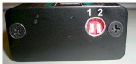
Figure 8 DIP switches and advance curve selection.
