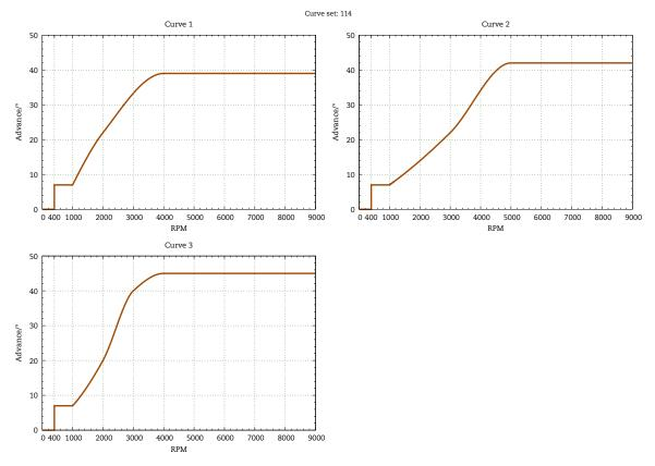
Figure 9 Selectable ignition curves.
