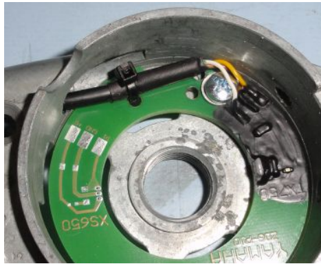
Figure 2 Mounting the pickup.
