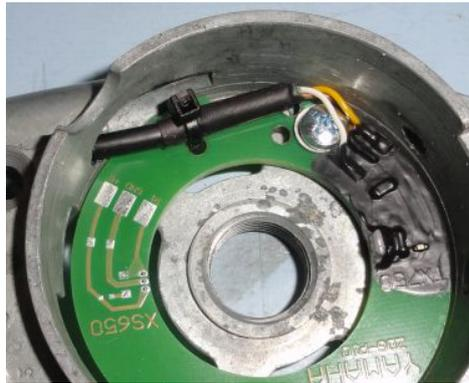
**Figure 2** Mounting the pickup.
