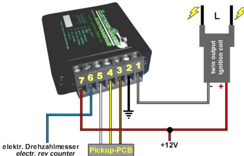
Figure 3 Circuit diagram.
