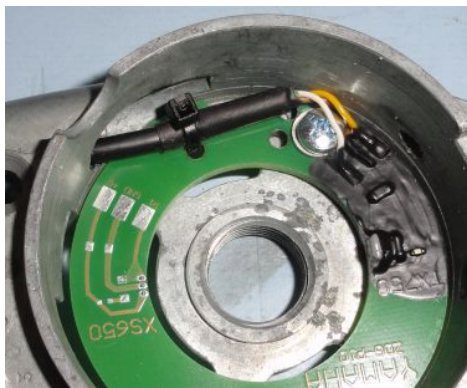
Figure 2 Mounting the pickup.
