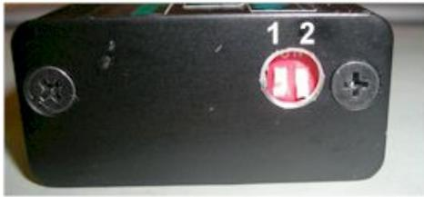
**Figure 8** DIP switches and advance curve selection.
