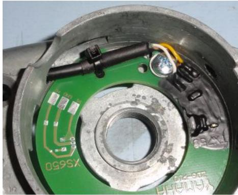
Figure 2 Mounting the pickup.
