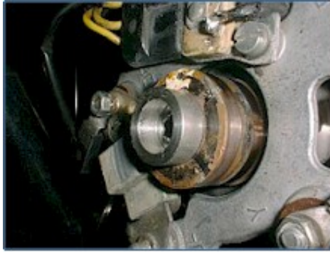
Figure 5.d Mounted driver sleeve
