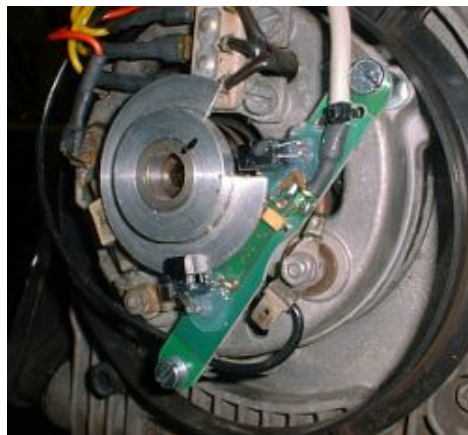
Figure 5.h Installed pickup and sector disk
