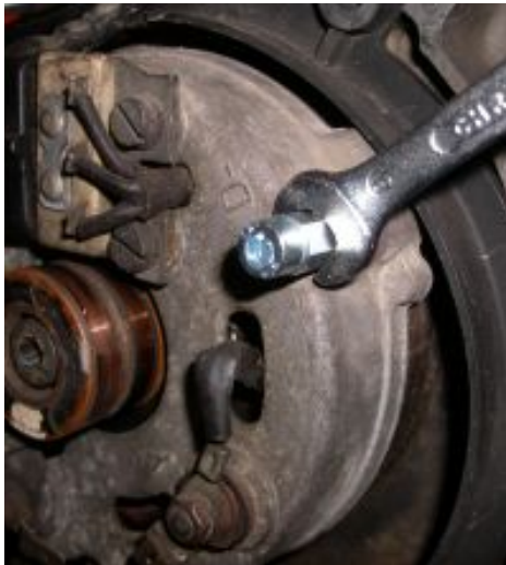
Figure 5.g Mounted spacer on the rods
