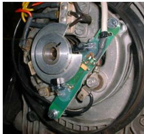
Figure 5 Installed pickup and sector disk
