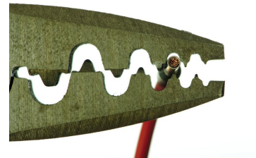
Using a professional crimp tool to crimp the ferrule.
