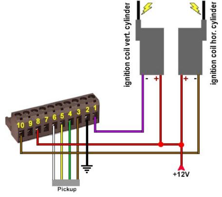
Figure 3 Connection diagram.
