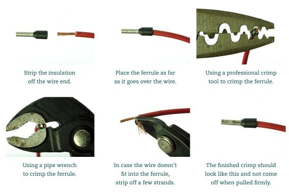
Figure 5 Crimping the wire end ferrules.
