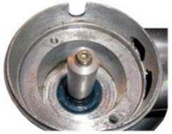
Figure 2 Mounting the driver sleeve on the shaft.
