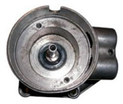
Figure 2 Removal of the old ignition components.
