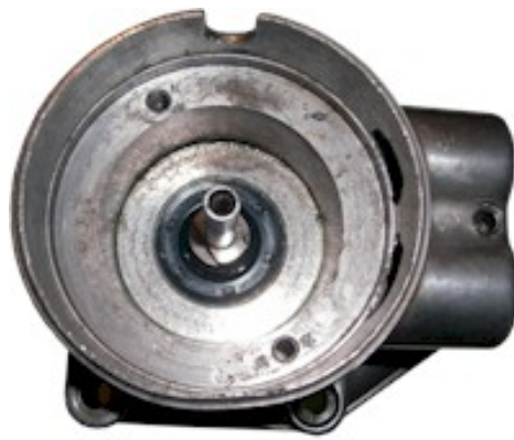
Figure 2 Removal of the old ignition components.
