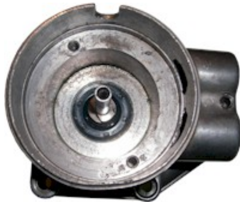
Figure 2 Removal of the old ignition components.
