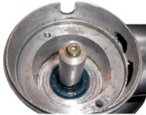
Figure 2 Mounting the driver sleeve on the shaft.
