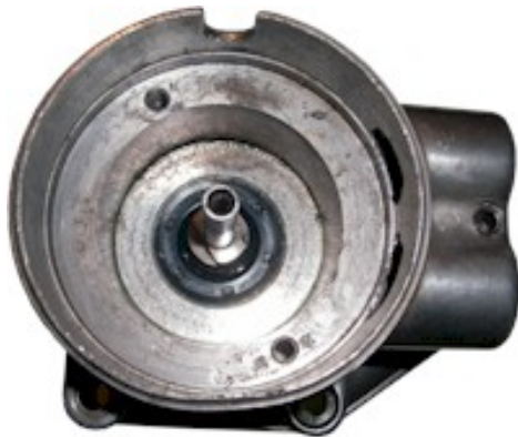
Figure 2 Removal of the old ignition components.
