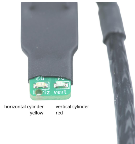
Figure 3 The red LED indicates the vertical cylinder, the yellow LED indicates the horizontal cylinder.
