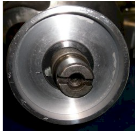
Magnet disk on the driver sleeve.
