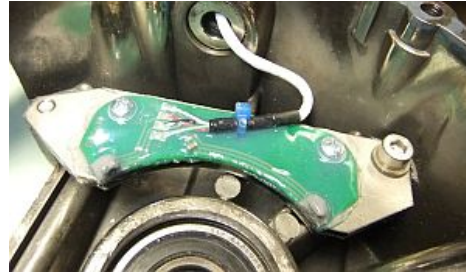
Mounting the pickup.
