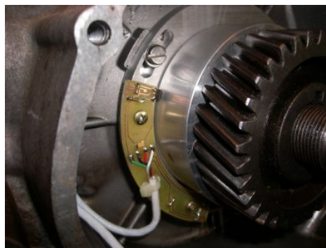
Mounting the new magnet disk on the primary gear.
